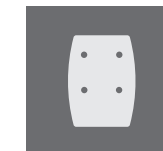
KLM-GD5068D/L150N Cut hole: L(177*177)*W50*H68mm
